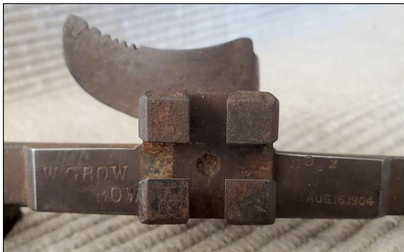
**Note the indentation in the center for seating the point of the thumb screw.**
